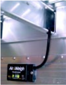
Fig. 1: Typical Trailer Installation without bracket
