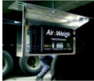
Fig. 2: Typical Trailer Installation using bracket
