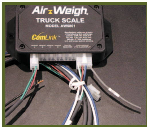
The suspension air pressure sensor is installed in the existing under-dash air gauge air line and the ComLink ECU is mounted out of the way under the dash.
